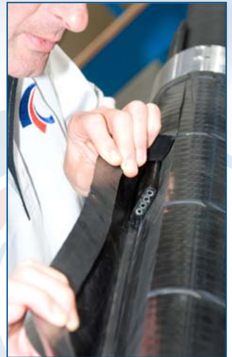
Make-up of control-line with the packer is extremely simple, and significantly reduces time and connections required when compared with mechanical packers
