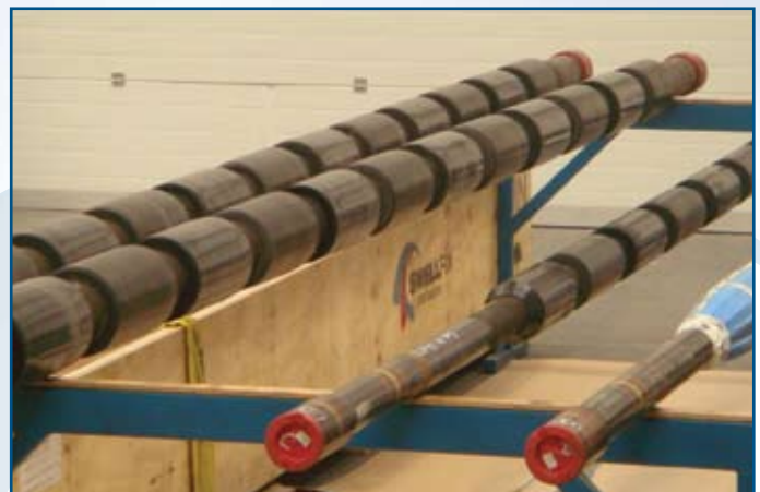
Packers banded design allow the Frac Isolation Packer™ to hold higher pressures in open hole applications
