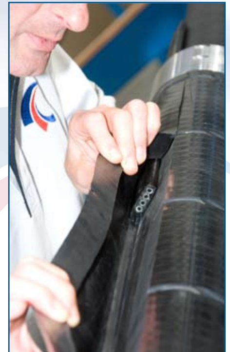
Make-up of control-line with the packer is extremely simple, and significantly reduces time and connections required when compared with mechanical packers
